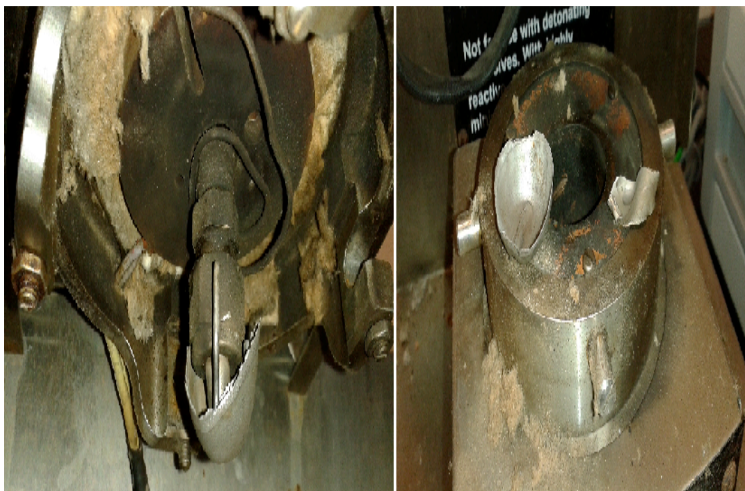
Figure 6: Photographs of the ARC equipment after test cell rupture.
