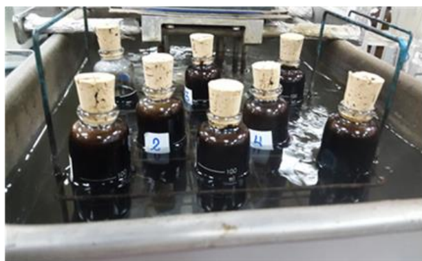
Figure A1: One-dimensional scans of pH and demulsifier concentration (180 °F, 14.7 psi).
