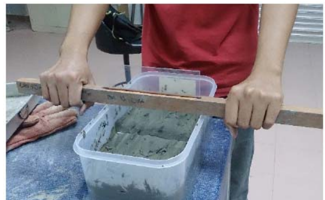
Figure 2: Smoothing of the bed's surface.
